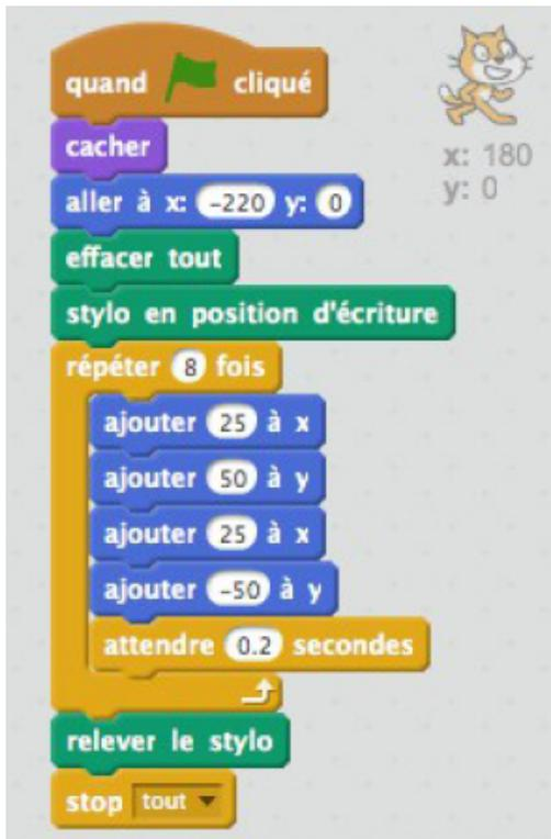
Scratch script for Exercise 1. The script starts with a 'when clicked' event block. It then performs the following actions: 'hide', 'go to x: -220 y: 0', 'erase everything', 'set pen to drawing', and a loop that repeats 8 times. Inside the loop, it adds 25 to x, adds 50 to y, adds 25 to x, adds -50 to y, and waits for 0.2 seconds. After the loop, it performs 'lift pen' and 'stop all'.
